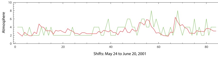
Fig. 3. Atmosphere during the first case period, May 24–June 20, 2001. Green/dashed gray: Experimental data; Red/solid black: prediction of U from the ANN in Fig. 2 with horizon = 1, computed according to (3.1).
