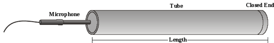
Figure 1: Experimental Setup for measuring the Speed of Sound
