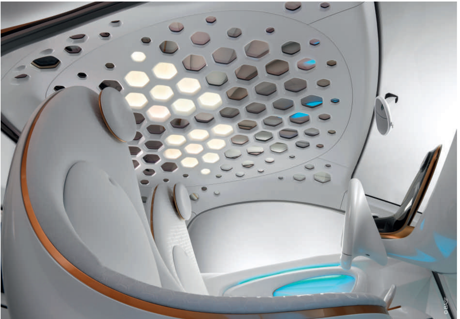
Transparent OLEDs create a spacious ambiance in the interior of the car.
