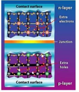
Although both materials are electrically neutral, n-type silicon has excess electrons and p-type silicon has excess holes. Sandwiching these together creates a: p/n junction at their interface, thereby creating an electric field.
