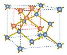
In the basic unit of a crystalline silicon solid, a silicon atom shares each of its four valence electrons with each of four neighboring atoms.
