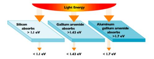
Different PV materials have different energy band gaps. Photons with energy equal to the band gap energy are absorbed to create free electrons. Photons with less energy than the band gap energy pass through the material.
