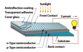
A typical solar cell consists of a glass or plastic cover, an antireflective coating, a front contact to allow electrons to enter a circuit, a back contact to allow them to complete the circuit, and the semiconductor layers where the electrons begin and complete their journey. The back contact of a cell—the side away from the incoming sunlight—is relatively simple. It usually consists of a layer of: aluminum or molybdenum metal.
