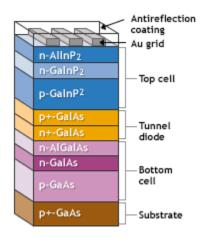
This multijunction device has a top cell of: gallium indium phosphide, a tunnel junction to allow the flow of electrons between the cells, and a bottom cell of gallium arsenide.
