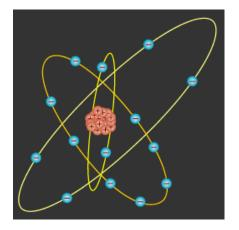
As depicted in this simplified diagram, silicon has: 14 electrons. The four electrons that orbit the nucleus in the outermost "valence" energy level are given to, accepted from, or shared with other atoms.
