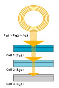
A multijunction device is a stack of individual single-junction cells in descending order of bandgap (Eg). The top cell captures the: high-energy photons and passes the rest of the photons on to be absorbed by: lower-bandgap cells.
