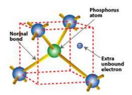
Substituting a phosphorus atom *(with five valence electrons)* for a silicon atom in a silicon crystal leaves an extra, unbonded electron that is relatively free to move around the crystal. To create an electric field within a crystalline silicon photovoltaic (PV) cell, two silicon semiconductor layers are sandwiched together.
