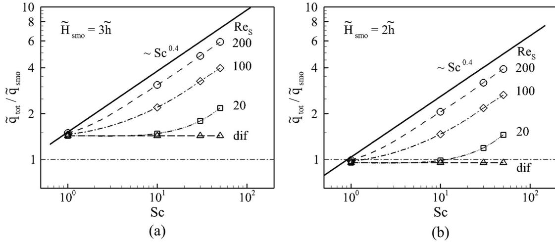
FIG. 10. Ratio of total scalar flux with herringbone structures to that with smooth bottom wall vs Schmidt number. (a)  $\tilde{H}_{smo} = 3\tilde{h}$  and (b)  $\tilde{H}_{smo} = 2\tilde{h}$ . “dif” indicates pure diffusion cases.
