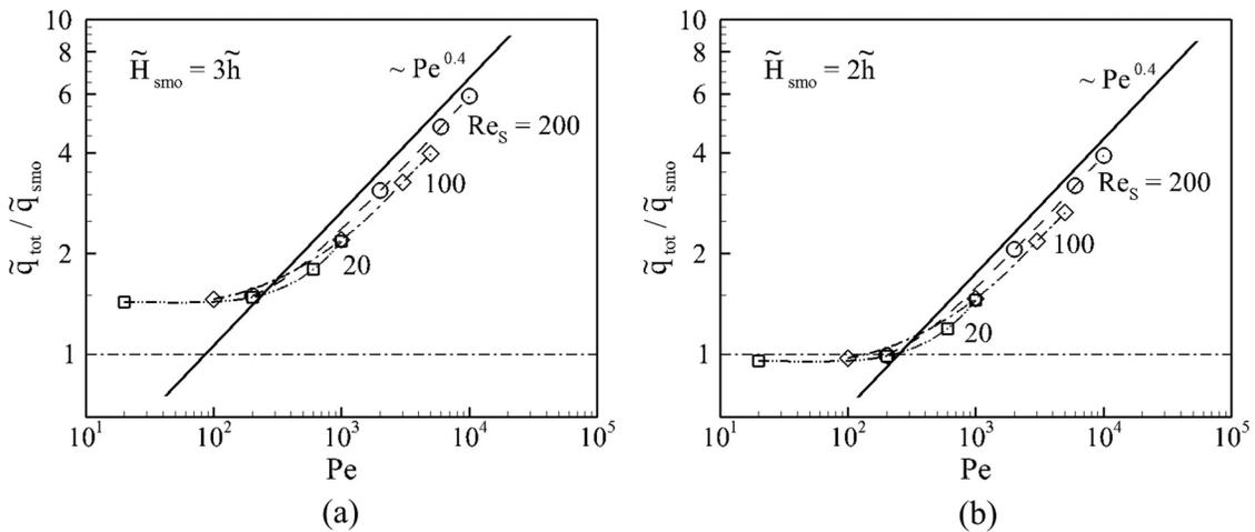
FIG. 12. Ratio of total scalar transport flux with herringbone structures to that with smooth bottom wall vs Peclet number. (a)  $\tilde{H}_{smo} = 3\tilde{h}$  and (b)  $\tilde{H}_{smo} = 2\tilde{h}$ .
