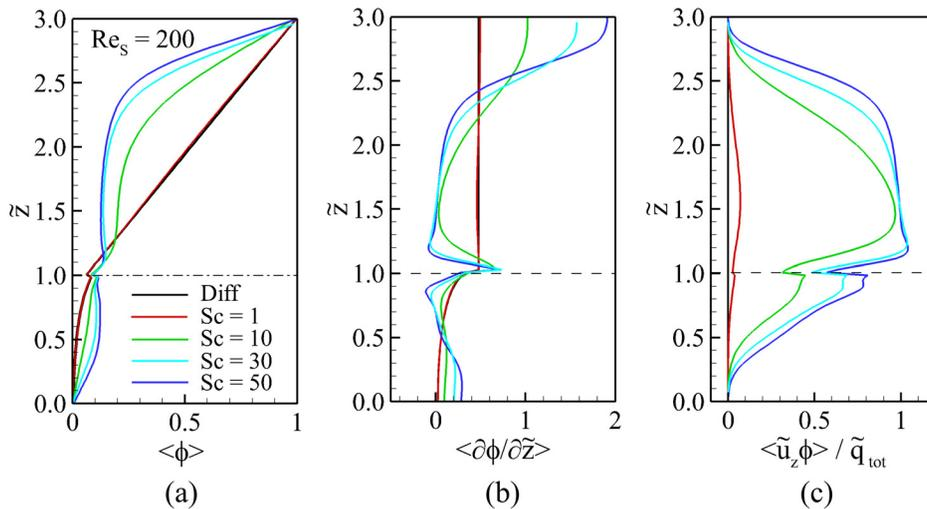
**FIG. 9.** Profiles of (a) horizontally averaged scalar concentration  $\langle \phi \rangle$ , (b) vertical gradient of scalar concentration  $\langle \partial \phi / \partial \tilde{z} \rangle$ , and (c) ratio of advective scalar flux to total scalar flux  $|\langle \tilde{u}_z \phi \rangle| / \tilde{q}_{tot}$  at  $Re_S = 200$ .
