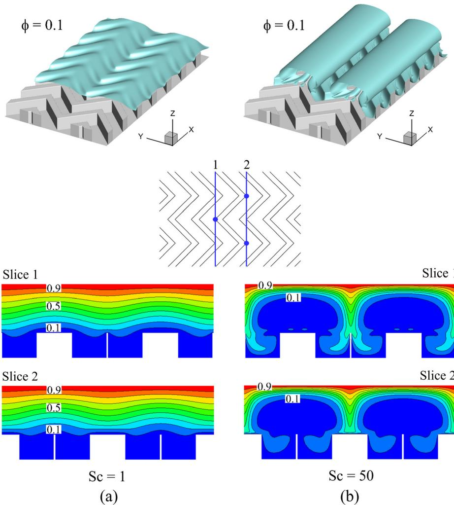
FIG. 6. Patterns of scalar concentration  $\phi$  at  $Re_S = 200$ . (a)  $Sc = 1$  and (b)  $Sc = 50$ . The sketch shows cross sections through the backward and forward connecting points of the grooves.
