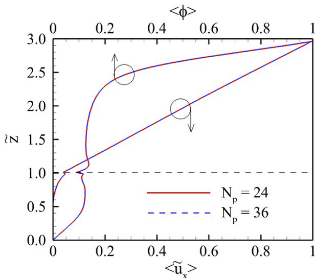
**FIG. 3.** Effect of grid resolution on horizontally averaged streamwise velocity ( $\langle \tilde{u}_x \rangle$ ) and scalar concentration ( $\langle \tilde{\phi} \rangle$ ) at  $Re_S = 200$  and  $Sc = 50$ .  $N_p$  is the number of grid points over one herringbone ridge.
