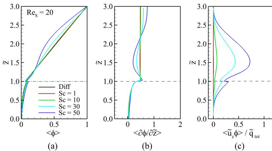
FIG. 8. Profiles of (a) horizontally averaged scalar concentration  $\langle\phi\rangle$ , (b) vertical gradient of scalar concentration  $\langle\partial\phi/\partial\tilde{z}\rangle$ , and (c) ratio of advective scalar flux to total scalar flux  $|\langle\tilde{u}_z\phi\rangle|/\tilde{q}_{tot}$  at  $Re_S = 20$ .
