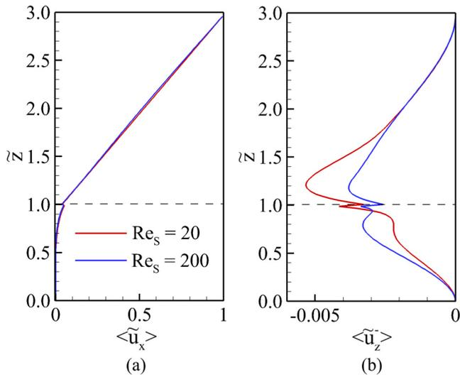
**FIG. 5.** Profiles of horizontally averaged velocity components. (a) Streamwise velocity  $\langle \tilde{u}_x \rangle$  and (b) effective downward velocity  $\langle \tilde{u}_z \rangle$ . The horizontal dashed line indicates the top of the herringbone ridges.
