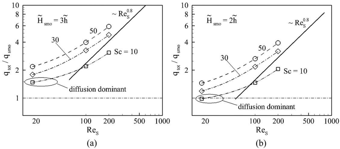
FIG. 11. Ratio of total scalar flux with herringbone structures to that with smooth bottom wall vs Reynolds number. (a)  $\tilde{H}_{smo} = 3\tilde{h}$  and (b)  $\tilde{H}_{smo} = 2\tilde{h}$ .
