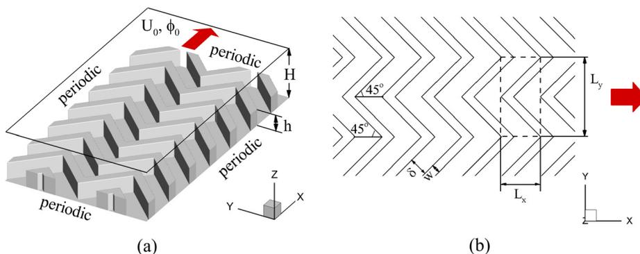
FIG. 1. Physical model of heat and mass transfer in a simple shear flow with herringbone structures on bottom wall. (a) 3D view and (b) top view. The dashed rectangle indicates the domain of numerical simulation.
