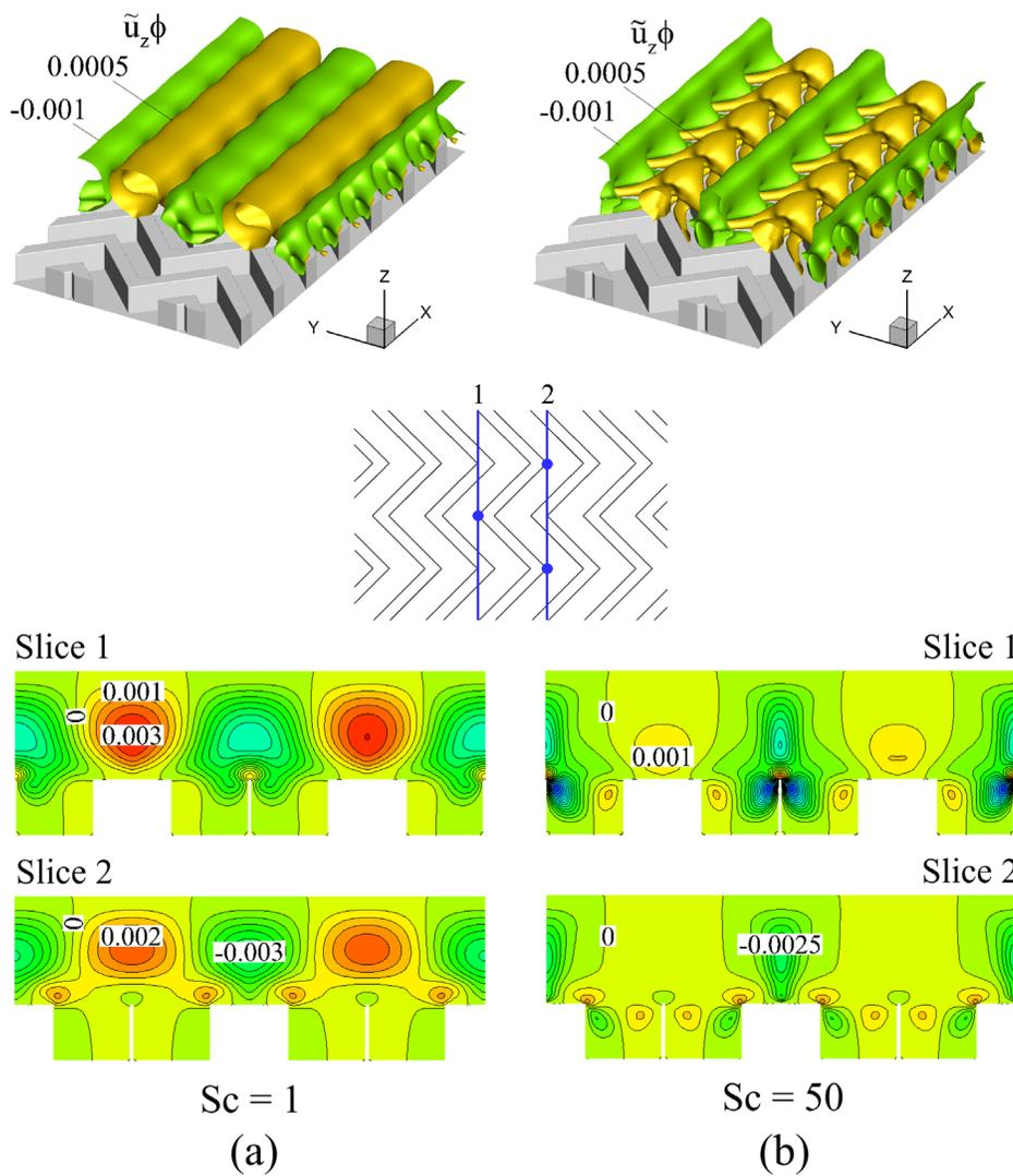
FIG. 7. Patterns of advective scalar flux in vertical direction  $\tilde{u}_z\phi$  at  $Re_S = 200$ . (a)  $Sc = 1$  and (b)  $Sc = 50$ . The slices are at the cross sections through the backward and forward connecting points of the grooves as shown in the sketch.
