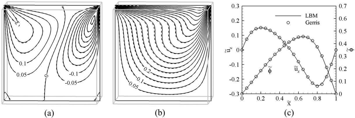
**FIG. 2.** Vertical velocity ( $\tilde{u}_z$ ) and temperature ( $\tilde{\phi}$ ) using the present LBM method (solid lines) and the open-source code Gerris (dashed lines). (a) Iso-contours of  $\tilde{u}_z$  on the middle  $xz$  plane, (b) iso-contours of  $\tilde{\phi}$  on the middle  $xz$  plane, and (c) profiles of  $\tilde{u}_z$  and  $\tilde{\phi}$  along the central streamwise axis.
